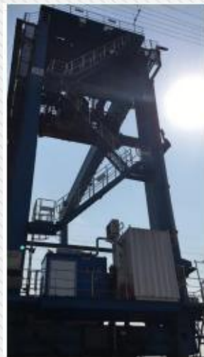
港口RTG: 62.7kWh (19S3P@2P12S)
