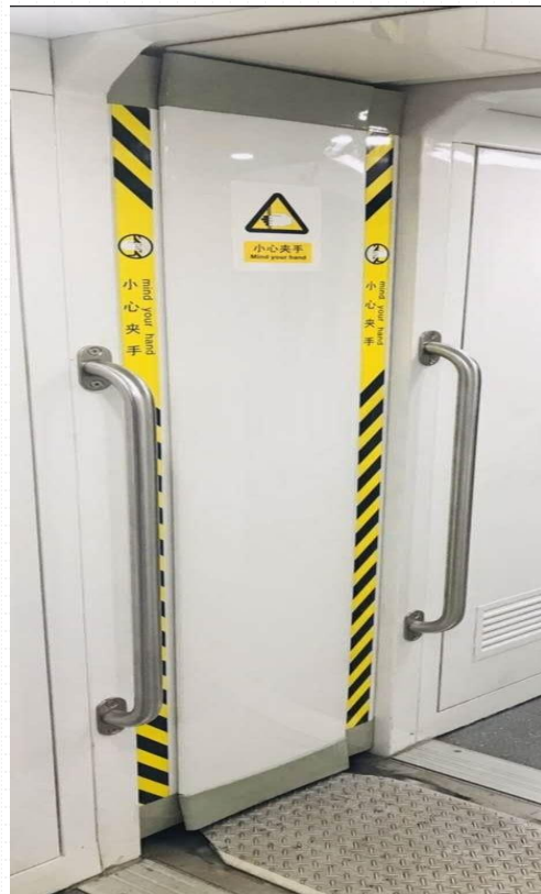
Three-piece guard plate for Type B cars
