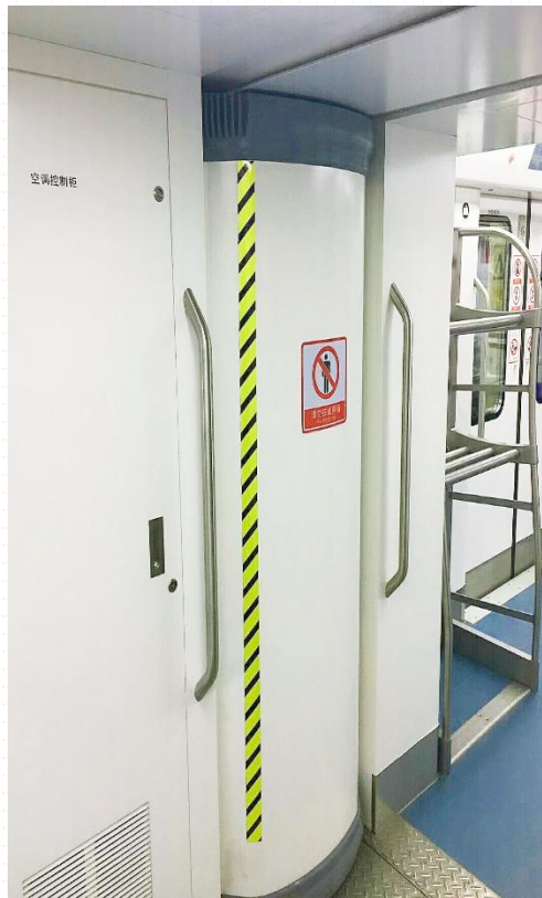
Type AS car has a one-piece guard plate
