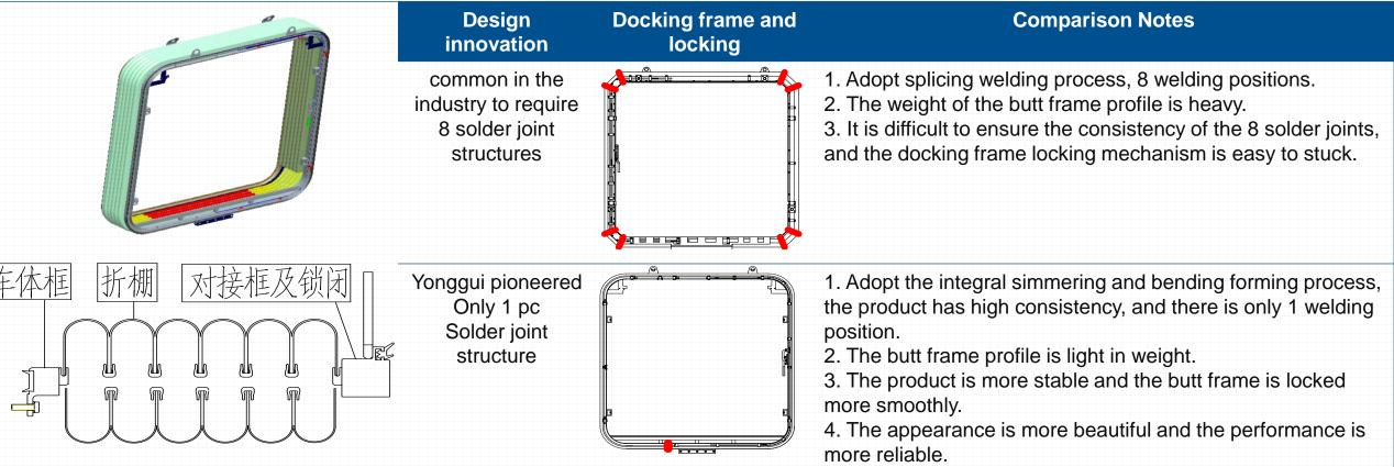
Optimize the docking frame and locking structure, the main highlights are as follows:
