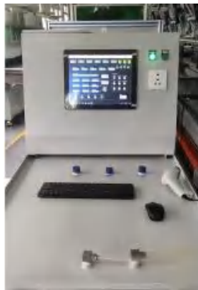
In-line Flow Rate Inspection for Liquid-cooled Charging Connectors
