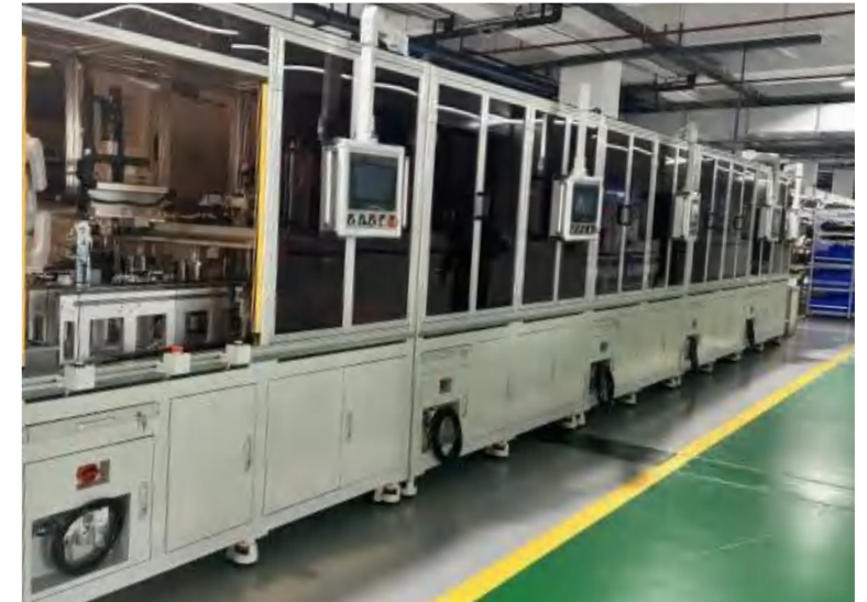
Automated Electronic Lock Production Line
