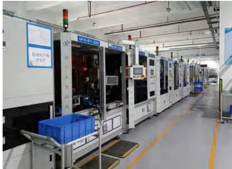
Automated AC Charging Connector Production Line
