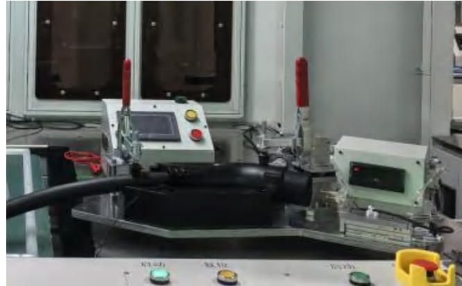
In-line Latch System Inspection
