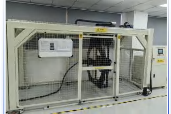
Cable Torsion Test Bench
