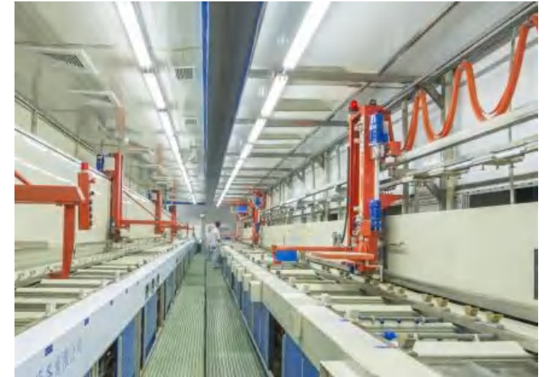
Automated Electroplating Production Line
