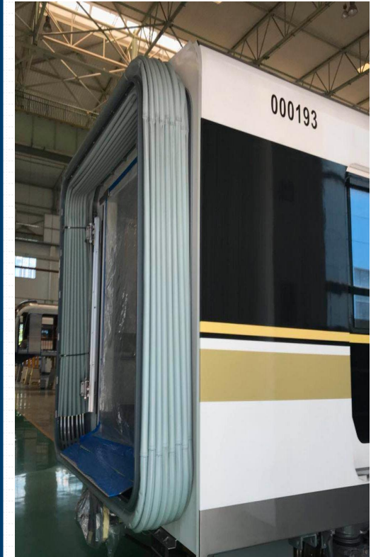
Chongqing Lines 4, 10 and Loop Line One-piece gangway for Type-AS vehicles
