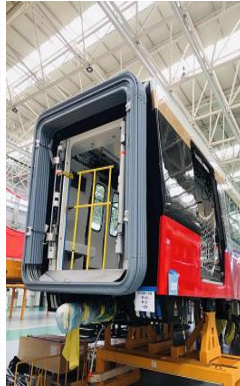
Xiamen Line 3, Shaoxing Line 1 One-piece gangway for Type-B vehicles
