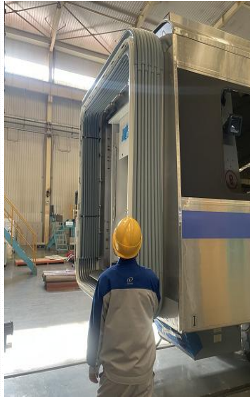
Hangzhou, Tianjin Beijing, Jinhua-Yiwu-Dongyang Three-piece gangway for Type-B vehicles
