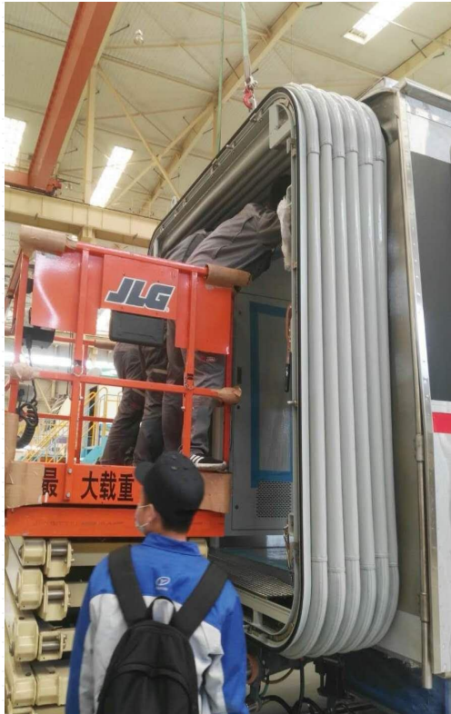
Taiyuan Line 2, Beijing Line 3 One-piece gangway for Type-A vehicles
