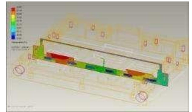
Sectional Temperature Nephogram
